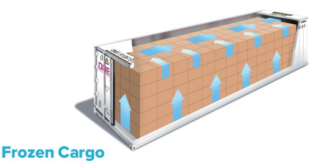
If frozen cargo is pre-cooled to the correct carrying temperature, it is only necessary for air to circulate around the periphery of the load. A block stow, i.e., one that has no deliberate spacing between any of the packages or pallets, is all that is required. However, it is necessary to ensure that air can circulate under, over and to each side and end of the stow.
