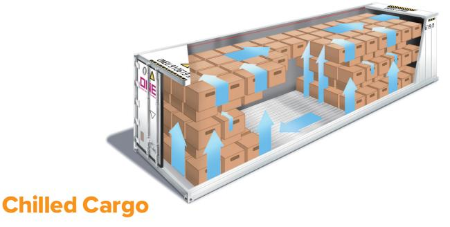
Chilled cargo is highly perishable premium food which can gradually ripen during shipment. In this illustration, the degree of air flow through the cargo is largely dependent upon the stuffing pattern at the door.
